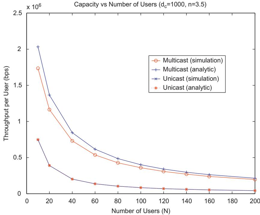
Fig. 1. Per user throughput for multicast and unicast schemes versus number of users. Path loss exponent is  $n = 3.5$ .
