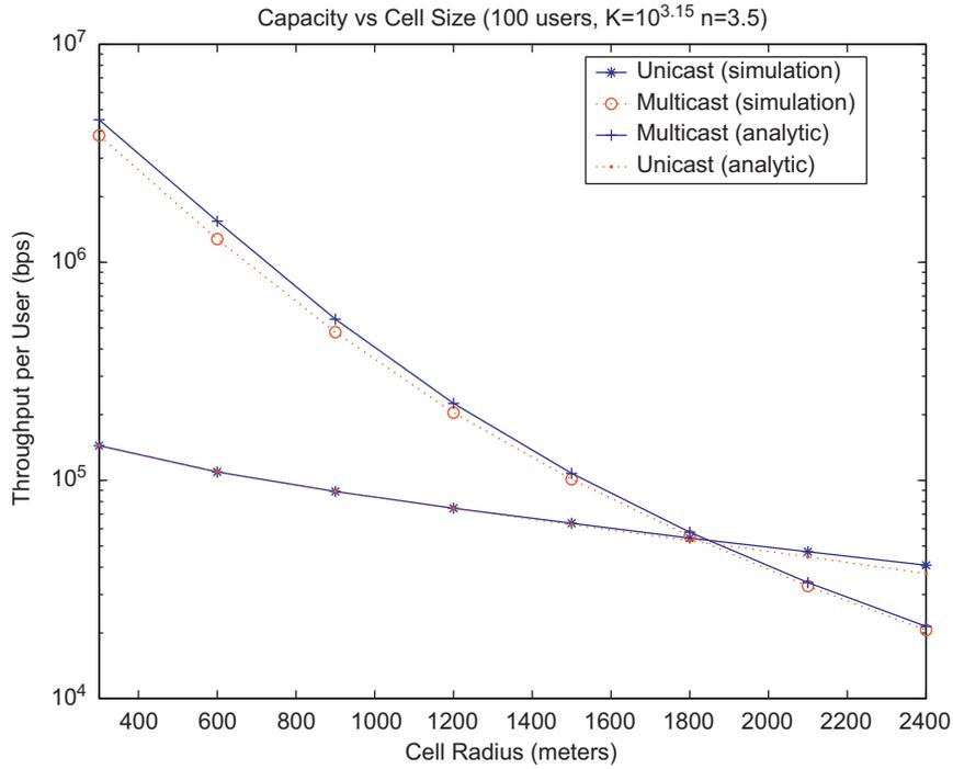
Fig. 2. Per user capacities for multicast and unicast schemes versus cell radius:  $K = 10^{3.15}$ ,  $n = 3.5$ .
