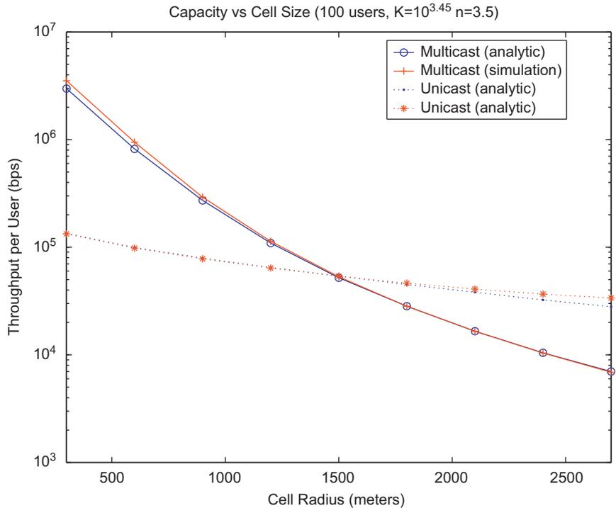
Fig. 3. Per user capacities for multicast and unicast schemes versus cell radius:  $K = 10^{3.45}$ ,  $n = 3.5$ .
