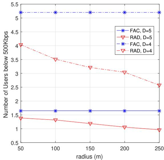
Fig. 5: Number of users having less than 500Kbps in transition mode.
