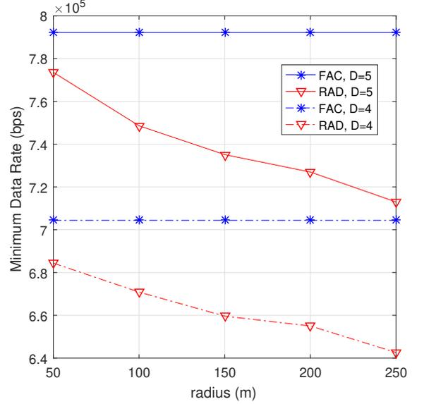
Fig. 3: Minimum user data rate in normal mode.
