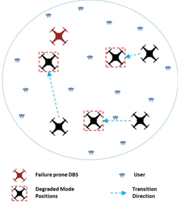
Fig. 1: System model of  $|\mathcal{D}| = 4$  DBSs deployed in normal mode. Transition mode starts after the DBS failure occurs. Remaining DBSs move along the direct path to their degraded mode positions minimizing the time spent for network recovery.
