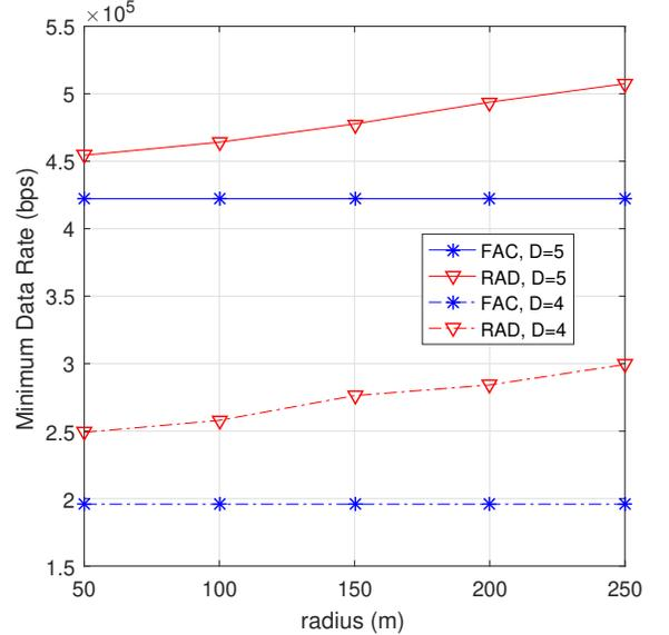
Fig. 4: Minimum user data rate in transition mode
